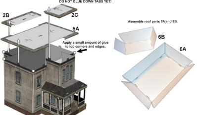
Apply a small amount of glue to bottom corners and top edges of roof parts 6A and 6B.
